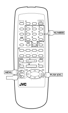
The G-code timer programming system eliminates the need to input channel, date, start and stop time data when setting the timer record function. Simply key in the G-code number for the TV programme you wish to record (found in most TV listings) and the recorder's timer is automatically programmed.
